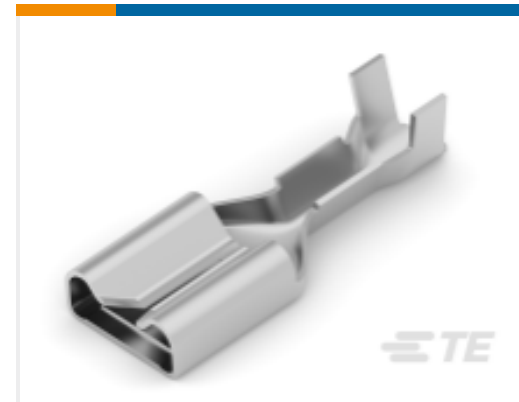
TE Part # 2238204-3 250 FASTON REC. 22-18AWG
